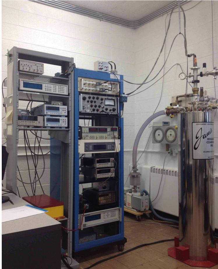
Figure 2.7: Equipment on the left shelf are LakeShore 370 AC resistance bridge, Princeton Applied Research P124A analog lock-in amplifier, SR 830 digital lock-in amplifier, EG&G 7265 digital lock-in amplifier, Keithley 2400 source meter, Keithley 2000 multimeter, CryoMagnetics CS-4 superconducting magnet power supply. On the right is the cryostat system.
