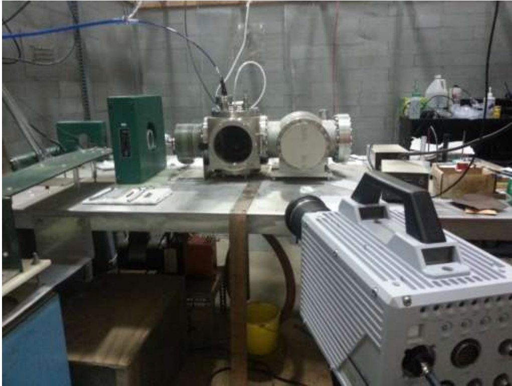
Figure 2.5: The blue fiber optic bundle from the spectrometer, top left, enters the top of the vacuum chamber. The plasma plume is recorded by the high speed camera, bottom right, through the viewport. Once charged, the capacitor in the bottom left of the picture is discharged to the source attached to the left of the chamber.
