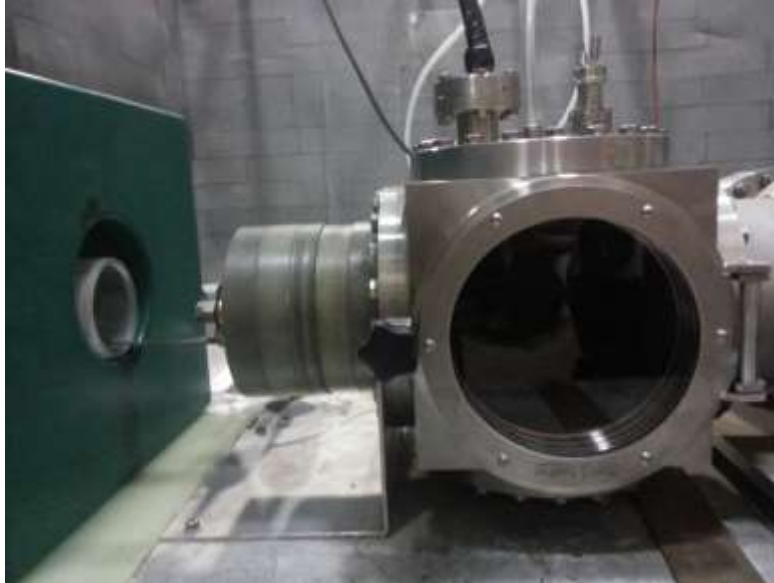
Figure 1.5: The electrothermal source is within the cylindrical insulator and bolted to the left side of the vacuum chamber to form a vacuum seal. It is bolted to the discharge power cable on the left, which passes through the Pearson coil to measure discharge current. The fiber optic cable for the spectrometer penetrates through the top of the chamber, and the quartz viewport in the front is for plasma viewing with the high speed camera
