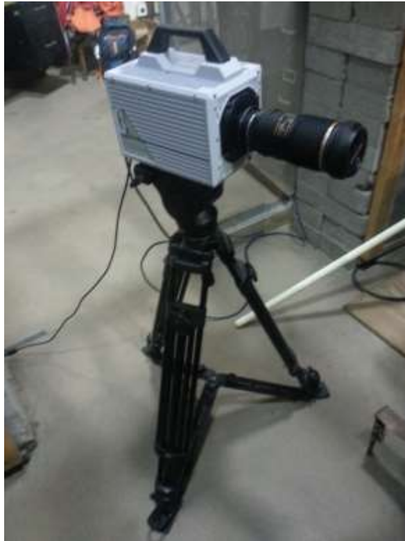
Figure 2.3: The FASTCAM SA4 high speed camera is mounted on a tripod to be level with the plasma plume as it exits the source. A 180 millimeter Nikon lens is used to obtain a close view of the ET discharge. The camera is placed away from the high voltage equipment to reduce electrical interference when in use.
