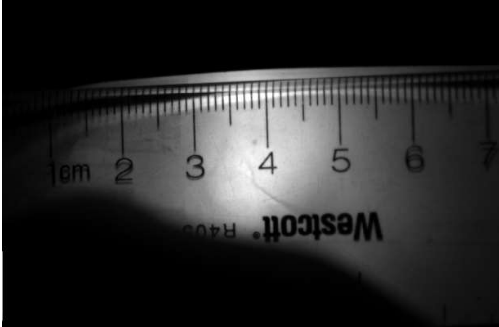
Figure 2.11: The calibration image, 1024x1024, was taken at the same focal length as the plasma video. The image is used to find the distance traveled by the discontinuity in the plasma video.
