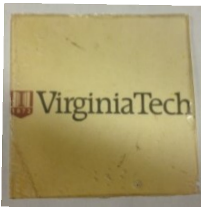
Figure 38. Film melt pressed at 190°C from an 82/18 PAN-co-MA.
