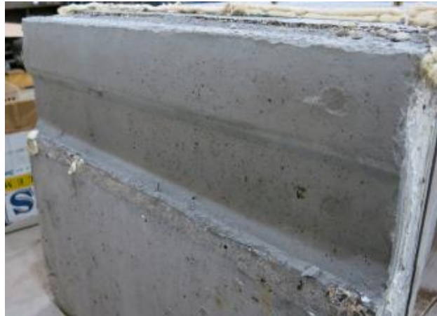
Figure 64: Picture of failed shear key of specimen 2 with no traces of bonded grout leftover
