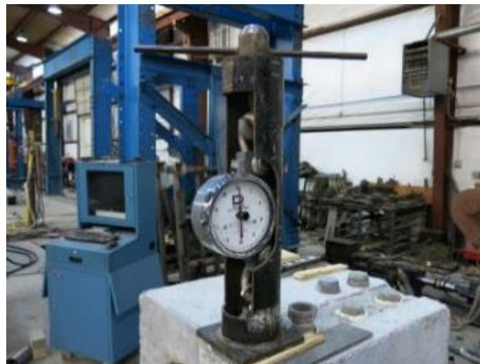
Figure 47: Picture of pull off test setup
