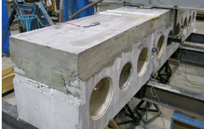
Figure 24: Picture showing concrete topping on top of sub-assembly.
