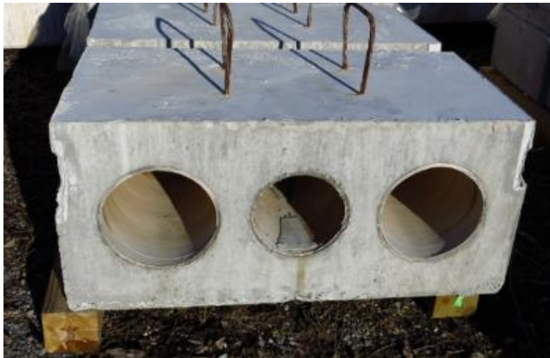
Figure 14: Finished Voided slab specimen
