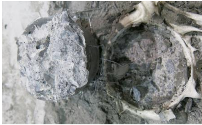
Figure 85: Picture of a VHPC pull off specimen with bonded concrete stuck to specimen
