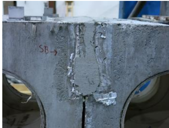
Figure 15: Hardened shear key from first specimen tested
