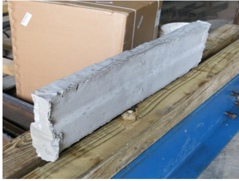
Figure 99: Fully intact shear key after failure of bonded connection
