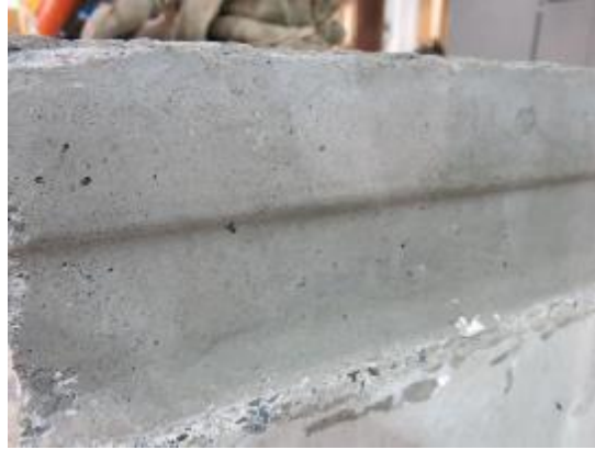
Figure 53: Shear key from middle section of the first specimen
