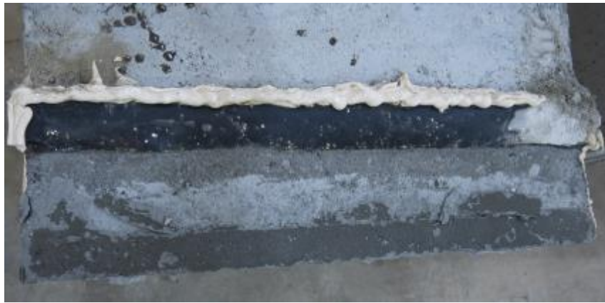
Figure 62: Picture of the middle section at the joint showing where the Kevlar debonded
