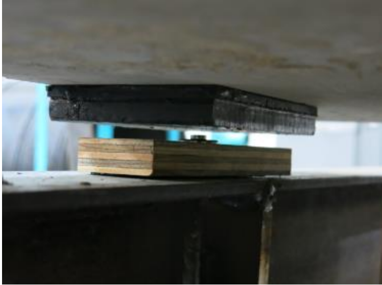
Figure 58: Uplift of south beam section at load cell
