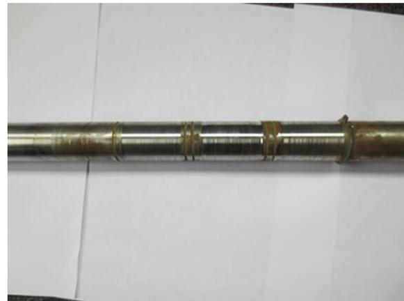
**FIGURE 9. MAIN DRIVE SHAFT FOR POLYMER BASED BEARING AFTER 60 HOURS OF TESTING [4]**
