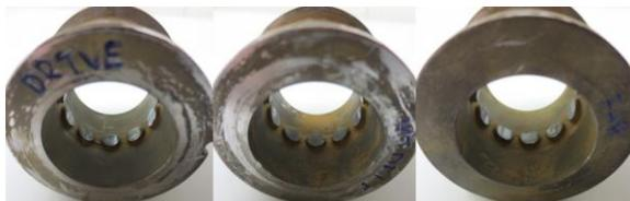
**FIGURE 14. THE LOAD (WORN) SURFACES OF PCD BEARINGS AFTER THE TEST. (A) DRIVE SIDE BEARING; (B) MIDDLE BEARING; (C) FAR SIDE BEARING.**
