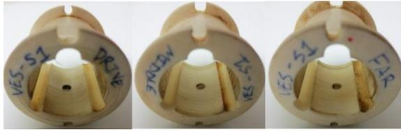
**FIGURE 11. THE LOAD (WORN) SURFACES OF VESCONITE BEARINGS AFTER THE TEST. (A) DRIVE SIDE BEARING; (B) MIDDLE BEARING; (C) FAR SIDE BEARING.**
