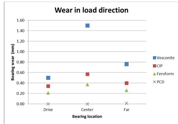
**FIGURE 8. WEAR OF CANDIDATE BEARINGS IN LOAD DIRECTION IN CLEAN WATER**
