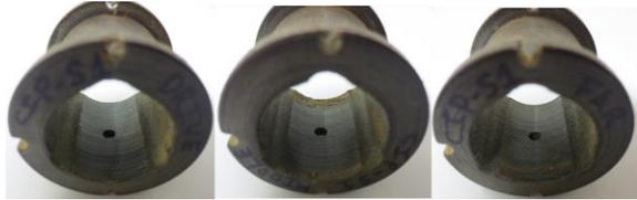
**FIGURE 12. THE LOAD (WORN) SURFACES OF CIP MARINE BEARINGS AFTER THE TEST. (A) DRIVE SIDE BEARING; (B) MIDDLE BEARING; (C) FAR SIDE BEARING.**
