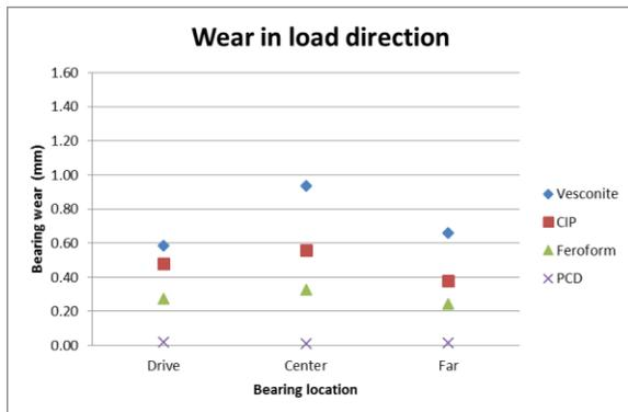
**FIGURE 7. WEAR OF CANDIDATE BEARINGS IN LOAD DIRECTION IN SEDIMENTED WATER**
