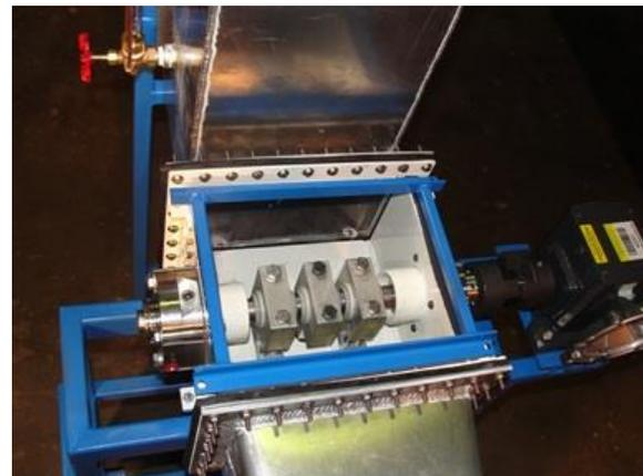
**FIGURE 2. ALL THREE BEARINGS MOUNTED ON THE FIRST STATION**
