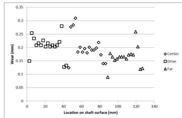
**FIGURE 10. WEAR VALUES ON (POLYMER BEARING) DRIVE SHAFT WITH RESPECT TO AXIAL SHAFT LOCATION (EXCLUDING SPLIT PIN AREAS BETWEEN TWO BEARINGS)**
