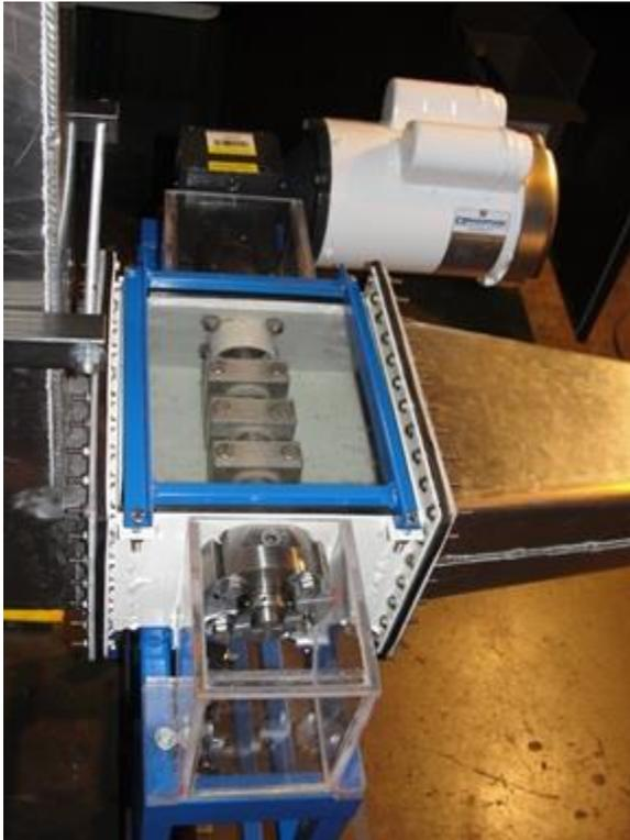
**FIGURE 3. FIRST STATION IS FILLED WITH CLEAN WATER AND BEARINGS ARE READY TO TEST; NOTE THAT PRESENT STUDY WAS CONDUCTED USING SEDIMENTED WATER, HOWEVER, CLEAN WATER FIGURE IS USED TO SHOW THE INSIDE COMPONENTS.**
