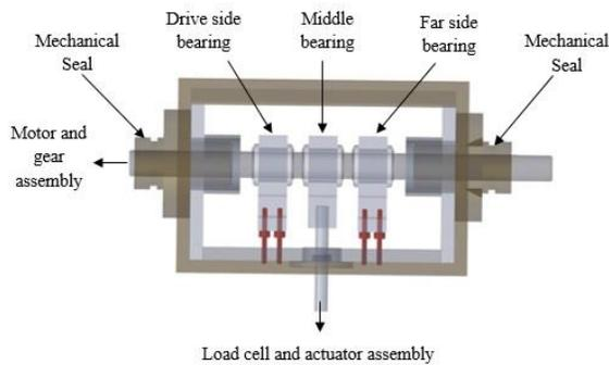
**FIGURE 4. THE CROSS SECTION OF A STATION**
