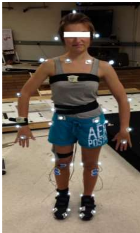
Figure 4. The picture of placement of reflective marker, inertial sensors and s-EMG
