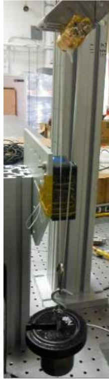
Figure 5.24: Static deflection test using laser displacement sensor to measure the deflection of the cable tie from an applied force due to hanging weight.
