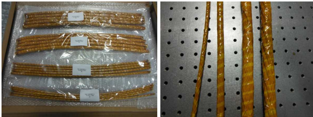
Figure 5.17: Samples of each of 1X7, 1X19, 1X48 and 7X7 spaceflight cables, in sets of five samples for each cable; single samples laid out to show uniformity of Kapton wrap.
