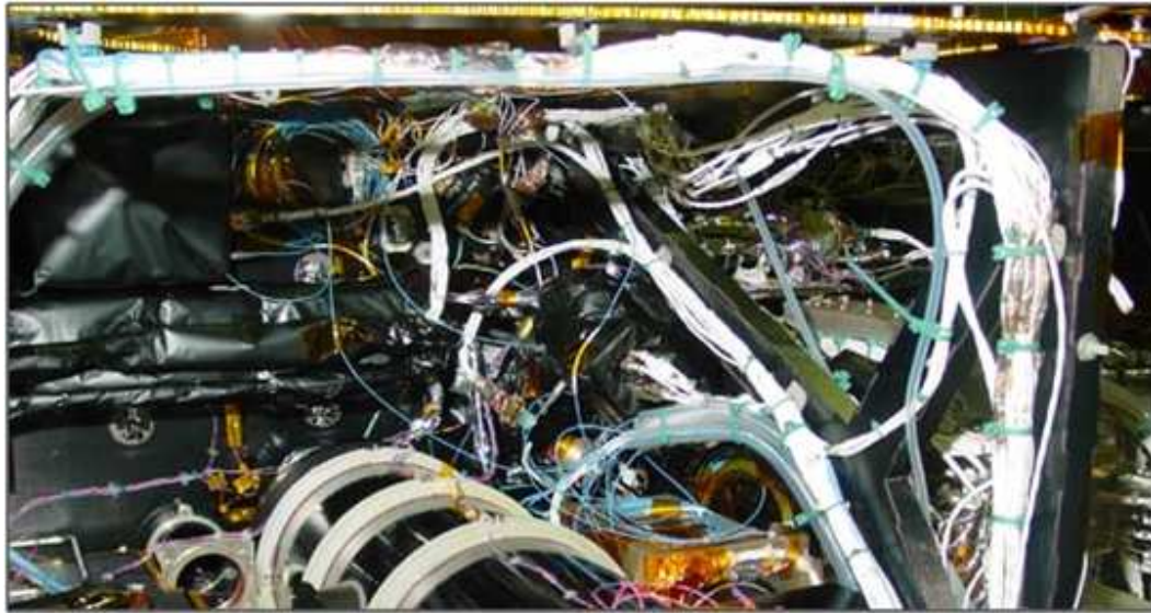
Figure 1.3: Cables and wires inside the ICESat spacecraft (assembled in 2002), showing the typical cable tie attachment method. Image courtesy NASA/Goddard Space Flight Center, public domain.
