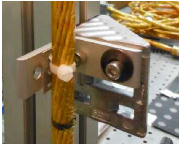
Figure 5.23: Cable secured to support via cable tie and TC105 tab.
