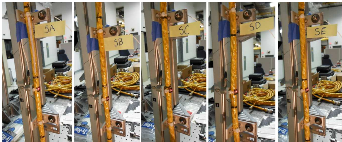
Figure 5.14: The five sections of 1x18 cable used for section comparison testing.
