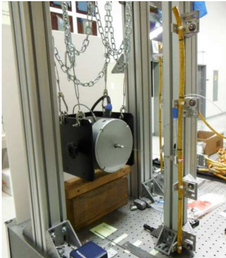
Figure 5.3: Preliminary cable testing of 1X18 test cable with suspended shaker.
