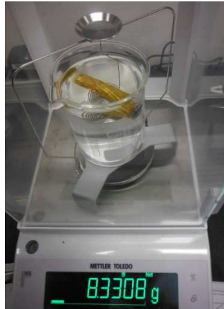
Figure 3.10: Cable in water for measurement of density based on Archimedes's principle of buoyant force.
