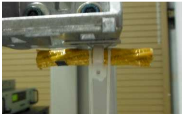
Figure 5.25: String harness for application of force for linear stiffness static and dynamic testing.
