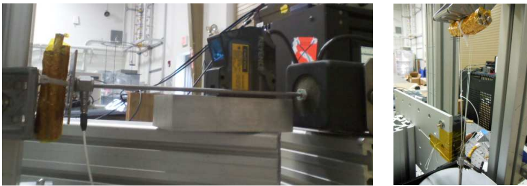
Figure 5.26: Test fixture iterations for dynamic testing of the attachment point linear stiffness.
