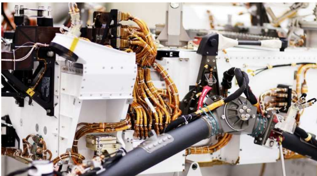
Figure 1.2: Kapton-wrapped cables on the Mars Rover "Curiosity". Photo copyright Joseph Linaschke, used with permission 1 .
