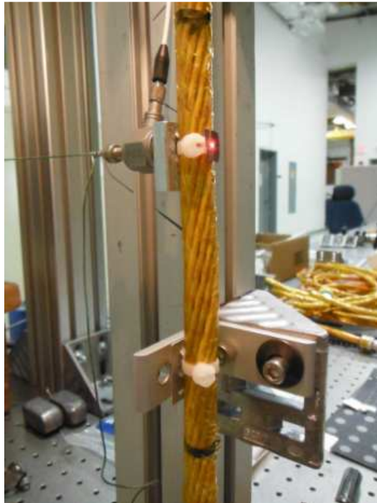
Figure 5.4: View of input force attachment method.
