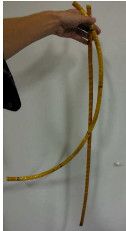
Figure 3.3: Evidence of inherent curvature in helical cable; in contrast, contra-helical cable hangs nearly straight.
