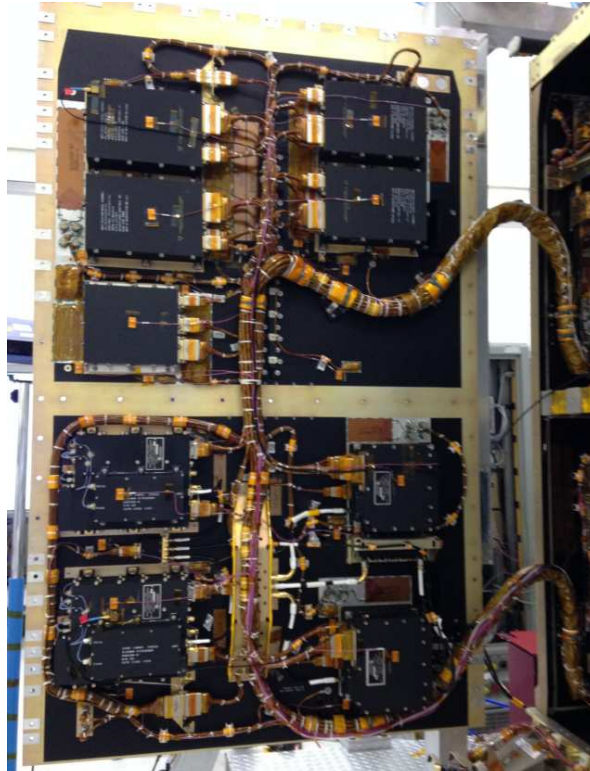
Figure 1.1: Cables of various sizes attached to an interior panel of the SMAP satellite due to launch in 2014. Image courtesy NASA/JPL-Caltech.
