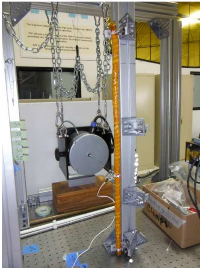
Figure 5.22: 1X48 cable in the two-point test fixture.
