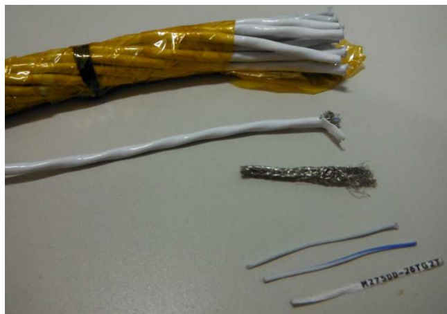
Figure 3.5: Deconstructed cable wire, from top to bottom; Kapton wrapped cable, individual wire, and wire components: EMI shield, two 26AWG twisted wire pairs, and wire filler label.
