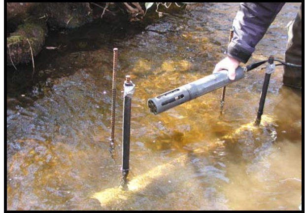
This probe contains sensors for continuous monitoring of water quality and depth.
