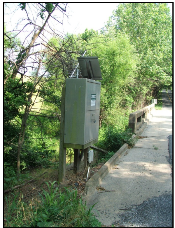
Stream-gaging station on North Fork Catoctin Creek near Waterford in Loudoun County, 6/25/10.
