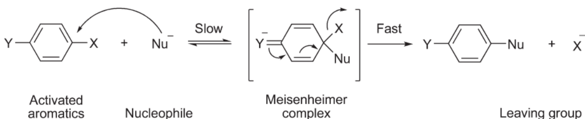
Figure 1.6: Mechanism of S_NAr nucleophilic aromatic substitution
