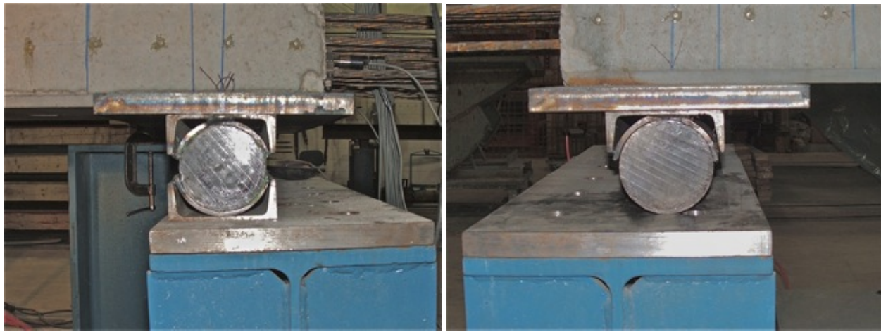
(a) (b) Figure 3-15. (a) Pin and (b) roller bearings.
