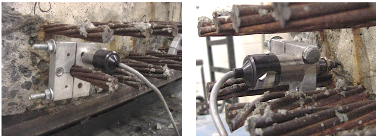
Figure 3-12. LVDT attached to end of prestressing strand for measuring slip during testing.
