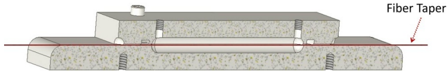
Fig. 4.2: Schemetic of the cross-section of a stop flow fixture.
