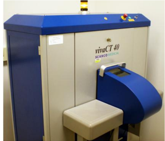
Fig. 1. Micro-computed tomography for the morphologic assessment of bone. The object of interest is placed in the center of the machine and a gantry, carrying the X-ray tube and detector, is rotated around it. X-rays produce cross-sectional images, or “slices”, which can be reconstructed into a three-dimensional image. These micro-CT units are located in the Institute for Critical Technology and Applied Science (ICTAS) Center for Biomedical Imaging at VA Tech.
