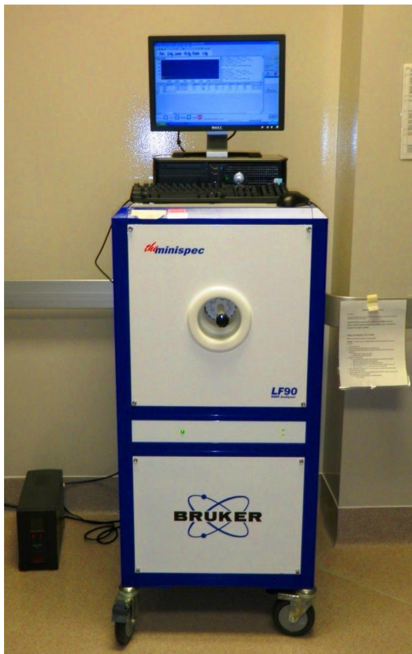
Fig. 2. Nuclear magnetic resonance for the evaluation of body composition.
