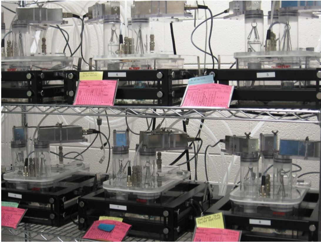
Fig. 3. Metabolic monitoring system to assess metabolic performance. Animals are maintained in their home cage which is outfitted with various monitoring devices that generate data on energy expenditure, physical activity, and water intake. This system is located in the Integrated Life Sciences Building (ILSB) at VA Tech.
