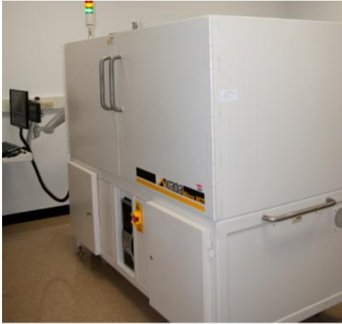
Fig. 1. Micro-computed tomography for the morphologic assessment of bone. The object of interest is placed in the center of the machine and a gantry, carrying the X-ray tube and detector, is rotated around it. X-rays produce cross-sectional images, or “slices”, which can be reconstructed into a three-dimensional image. These micro-CT units are located in the Institute for Critical Technology and Applied Science (ICTAS) Center for Biomedical Imaging at VA Tech.
