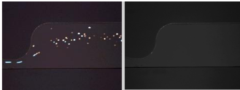
Figure 19: One, of 20 randomly selected, input frame used for calculating the background image using a median filter on left and resultant background image on right.
