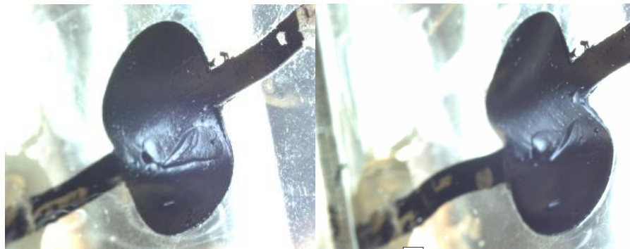
Figure 49: The micropump buckles when voltage is applied. Left shows the micropump when no voltage is applied and there is no buckling. Right shows the amount of buckling that occurs when 12kV are applied.
