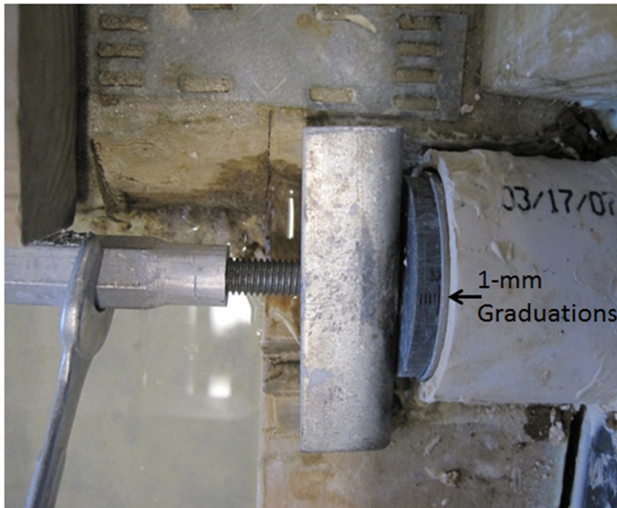
Figure 3.2 Sample support bracket and advancer with graduation markings used to advance soil sample and track erosion
