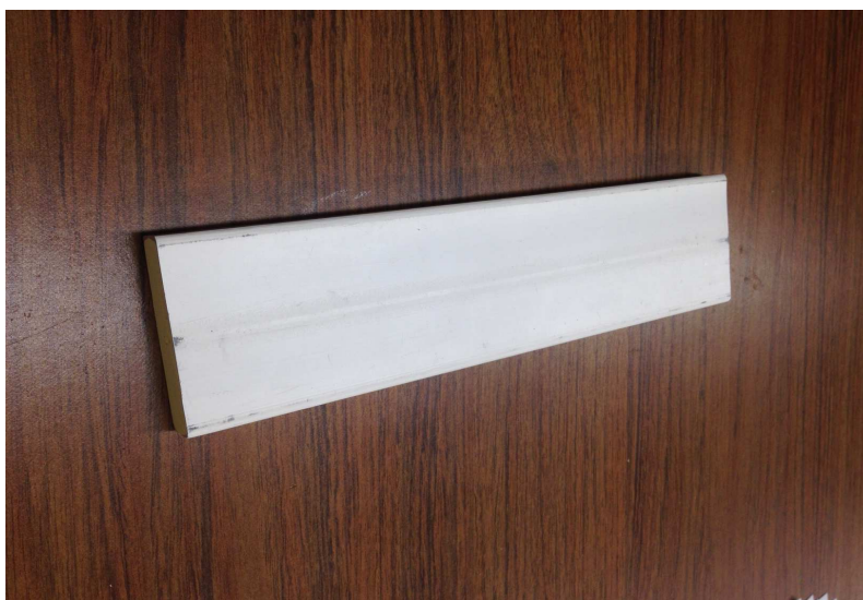
Figure 3.3: A photo of a strip with the white \text{TiO}_2 coating visible.
