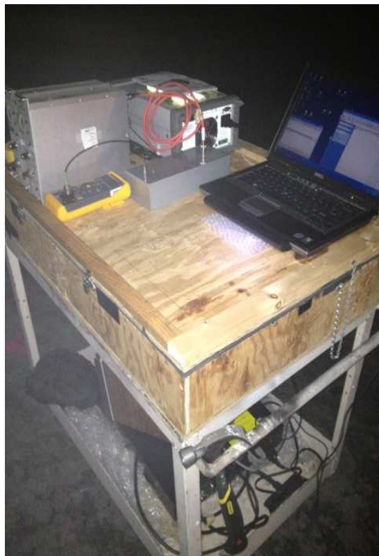
Figure 3.10: The box containing the detector with the laptop, HV and LV modules on top.
