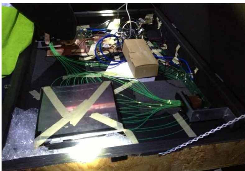
Figure 3.11: The detector inside the box. The green fiber optic cables are visible that connect the strips to the MAPMTs.
