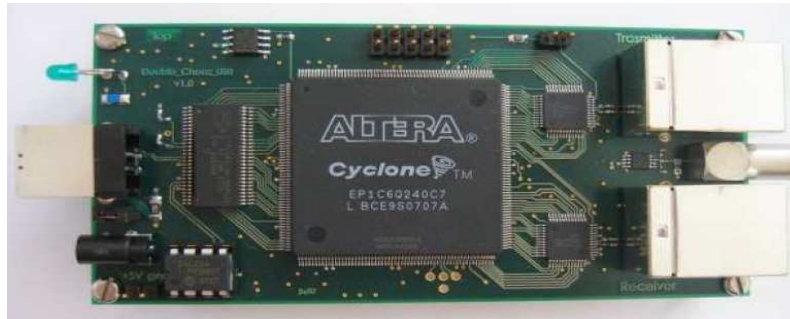
Figure 3.9: A picture of the USB board with the Altera FPGA.
