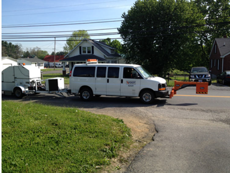
Figure 15. FWD and GPR Testing Equipment
