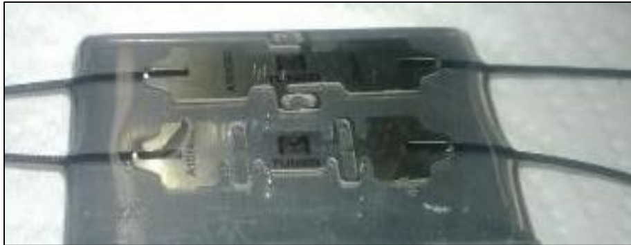
Figure 3.10 Epoxied temperature sensor and strain gage on Al 3003 substrate.
