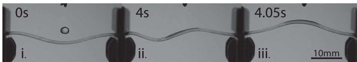
Figure 4.1: Swelling induced snap buckling of a clamped Polydimethylsiloxane (PDMS) arch.
