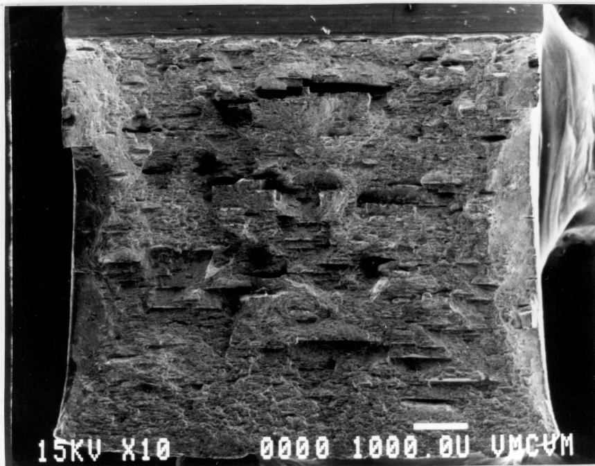
Figure 27. Fracture surface of a rolled-plate, liquid nitrogen impact test, 10X.
