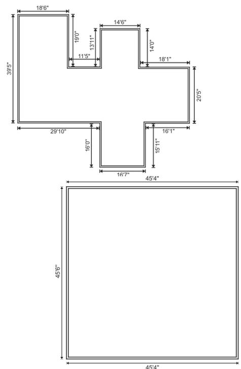
The narrowest parts of the home should be exposed to the east and west (see below). In other words, for optimum efficiency the home should be oriented so that its long axis runs from east to west. This reduces the total amount of surface area exposed to the summer sun, yet when needed in cooler regions, allows the low-angle rays of the winter sun to warm the southern exposure (free solar heating).
