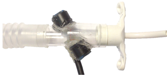
Figure 5-16: AT300 transducers shown embedded in the final sensor flow chamber, which is attached to a respiratory tube and neonatal tracheostomy tube
