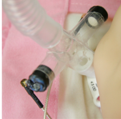
Figure 4-4: Second-generation prototype sensor connected to a doll with tracheostomy tube
