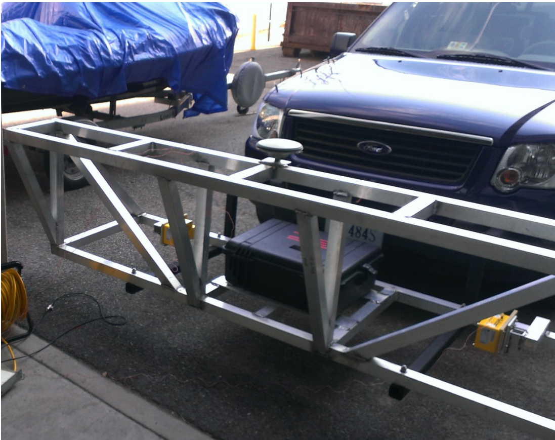
Figure 19: This shows the normal data taking setup of the equipment frame. The two yellow Roline lasers are seen on the sides in the wheel track. The black Pelican case in the middle houses the IMU and GPS receiver, while the circular GPS antenna is on the top of the frame.
