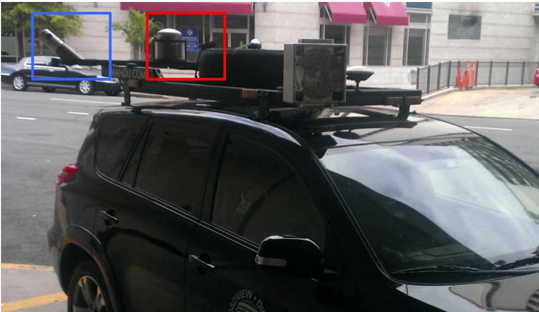
Figure 11: A road profiling system. The INS is in the red box, and a sensor is in the blue box. Note they are connected by a relatively thin piece of metal. Photo by author, 2014.
