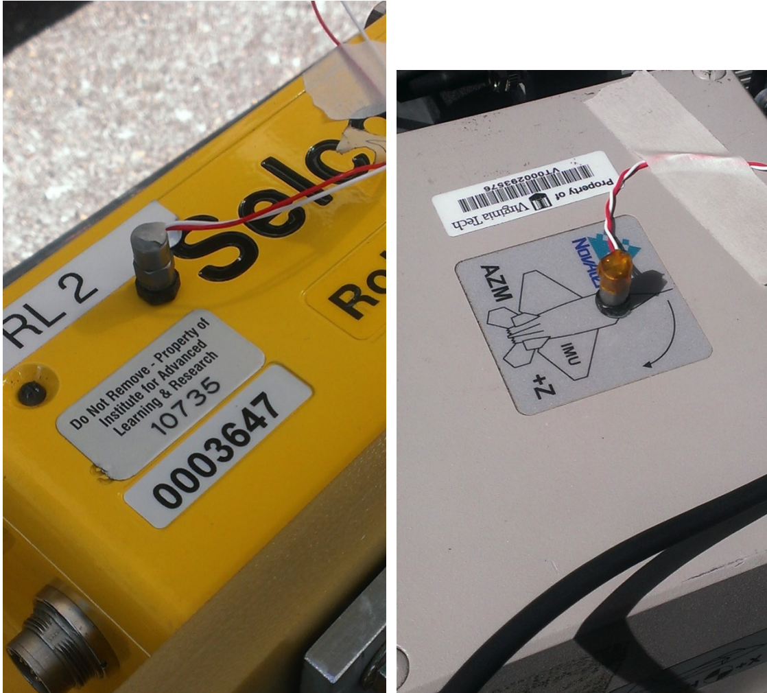
Figure 20: This shows the accelerometers attached to the Roline laser (left) and IMU (right).
