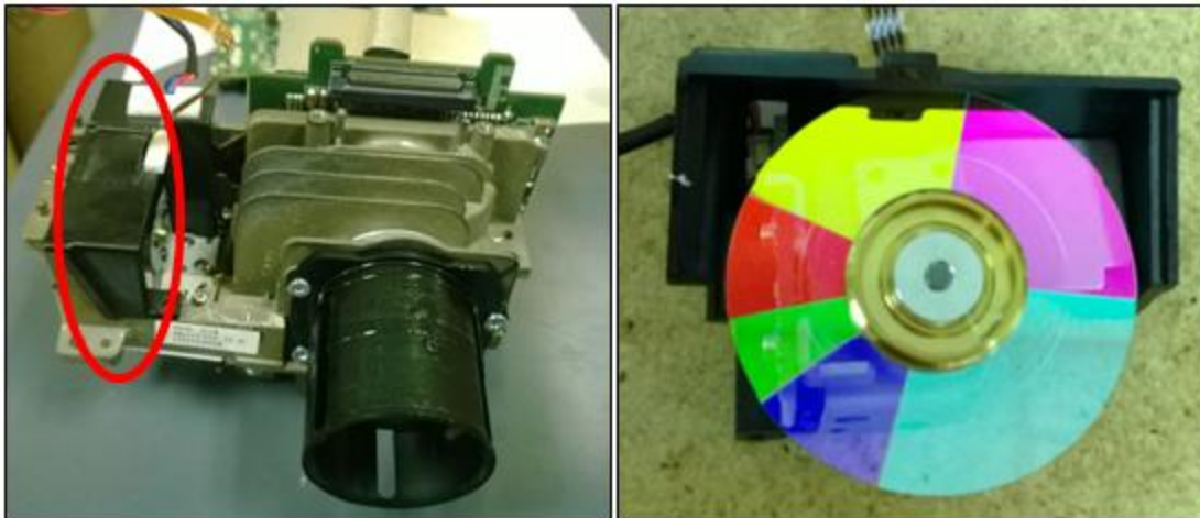
Figure 3-7. The color wheel and bandpass filter are located in the projector’s optical engine and identified by the red circle. Access to these components requires full disassembly of the projector.
