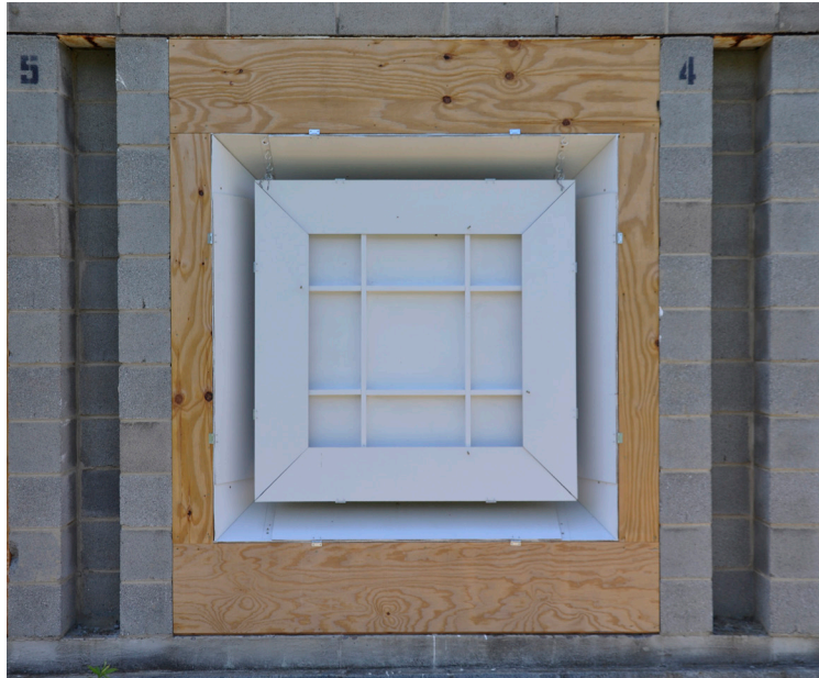
Light reflectors in closed position
