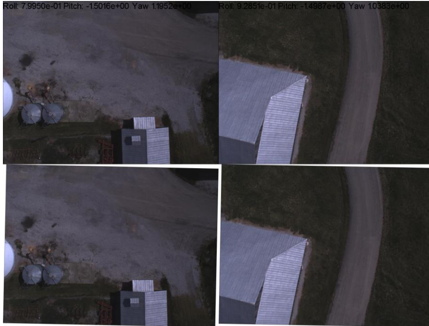
Figure 39: Images were transformed based on IMU information to closely approximate a nadir view for image mosaicking. Photos by author, 2014.
