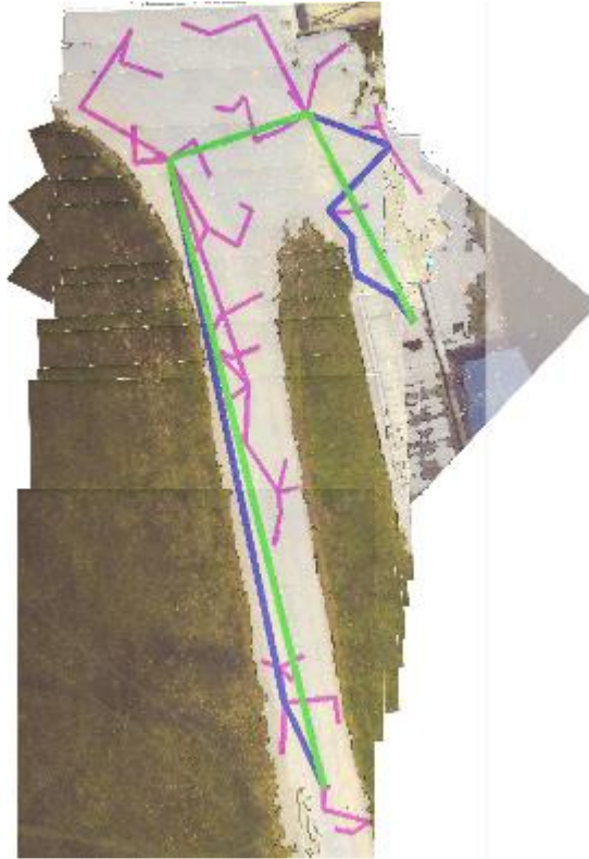
Figure 48: A simple test incorporating all facets of the developed algorithm shows the robustness of the algorithm to data without calibrating parameters. The images are still effectively mosaicked, road detection and path planned for a ground vehicle. Photos by author, 2014.
