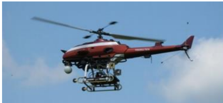
Figure 37: The Yamaha RMX UAV is used for many different missions for the USL and has captured aerial imagery that can be analyzed for these algorithms. Photo by author, 2014.
