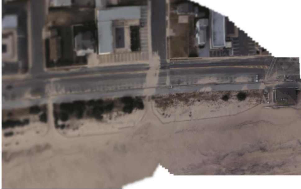
Figure 15: Image mosaicking with dynamic cropping shows a traveling window to remove less recent data for easier mosaicking. Newest image is in the bottom right, and blurring is due to averaging since images to the left are older [29] [National Oceanic and Atmospheric Administration, "Hurricane SANDY Response Imagery," National Geodetic Survey, 2012]. Used under fair use, 2014.
