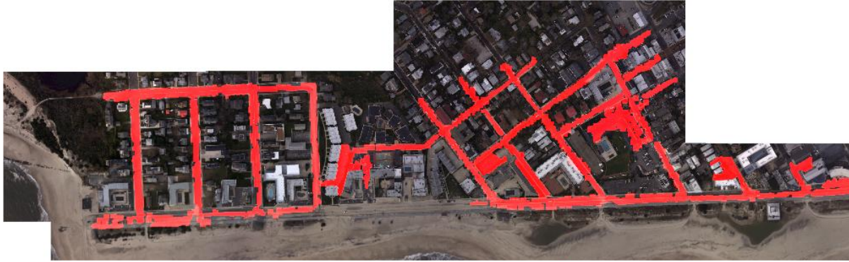
Figure 26: Final large map created from continuous mosaic and road detection algorithms. Areas selected correspond to determined road locations [National Oceanic and Atmospheric Administration, "Hurricane SANDY Response Imagery," National Geodetic Survey, 2012]. Used under fair use, 2014.
