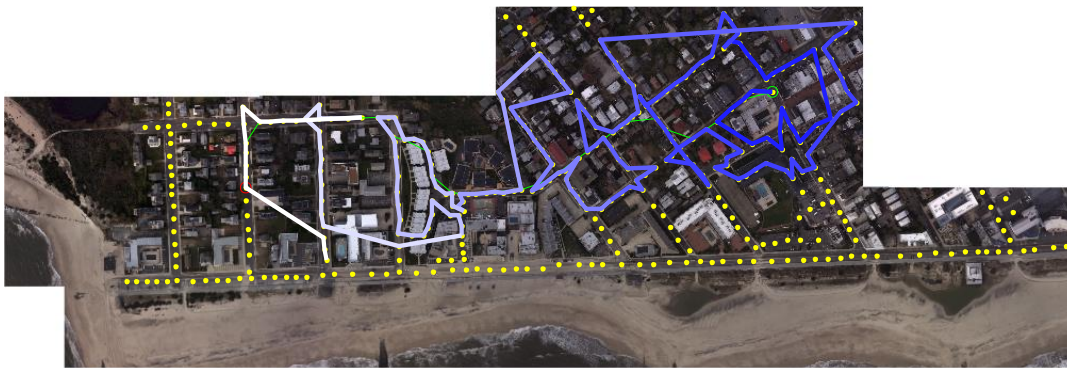
Figure 30: A flight path (blue-white line) determined in order to map areas with an aerial vehicle using a TSP genetic algorithm with a traveling wave applied to prioritize locations based on distance [National Oceanic and Atmospheric Administration, "Hurricane SANDY Response Imagery," National Geodetic Survey, 2012]. Used under fair use, 2014.
