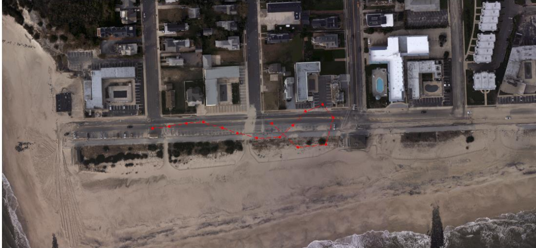
Figure 13: Sample flight plan for simulated images based on a larger resolution image and taking sample images at and between the given points (red). [National Oceanic and Atmospheric Administration, "Hurricane SANDY Response Imagery," National Geodetic Survey, 2012]. Used under fair use, 2014.
