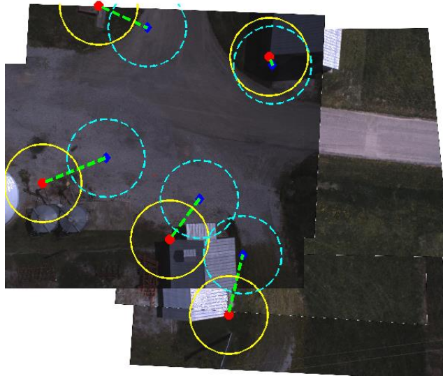
Figure 46: GPS ground truth points (red) were compared to calculated GPS locations (blue) from geo-tagged images (uncertainty shown). Distances measured between points show an average error around 15 feet. Photos by author, 2014.
