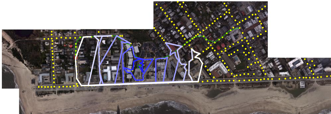
Figure 31: This figure shows how the TSP Traveling Wave algorithm can be re-run to determine a new flight plan (blue-white line) when the area mapped is insufficient [National Oceanic and Atmospheric Administration, "Hurricane SANDY Response Imagery," National Geodetic Survey, 2012]. Used under fair use, 2014.
