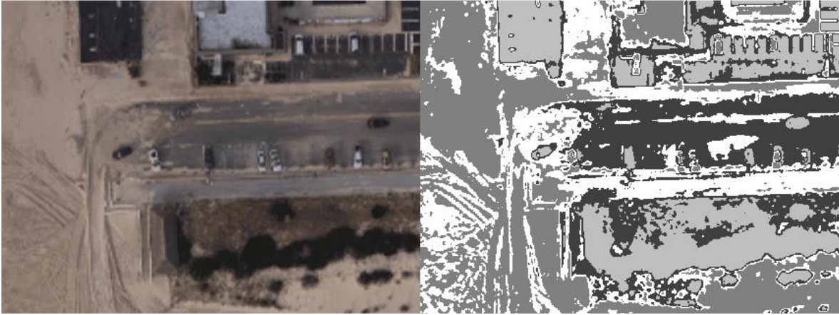
Figure 17: K-means (4 centers) image clustering performed on a single image based on RGB values [National Oceanic and Atmospheric Administration, "Hurricane SANDY Response Imagery," National Geodetic Survey, 2012]. Used under fair use, 2014.
