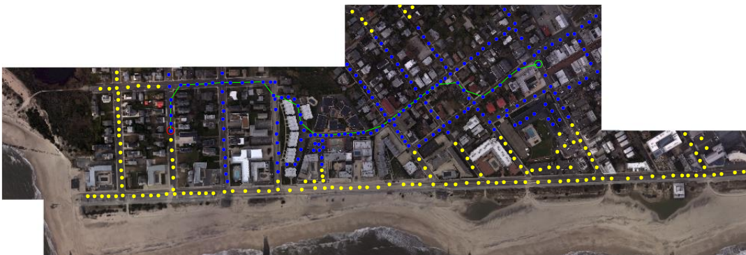
Figure 28: All points in blue were selected for mapping purposes. They are currently determined by Dijkstra's algorithm for shortest path (shown in green) and a given distance from a vector between
