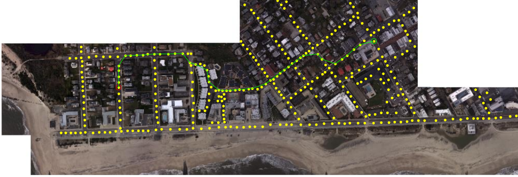
Figure 27: A set of known road points on a given map with Dijkstra's algorithm calculating the shortest path. This can be used to prioritize mapping locations for the UAV [National Oceanic and Atmospheric Administration, "Hurricane SANDY Response Imagery," National Geodetic Survey, 2012]. Used under fair use, 2014.
