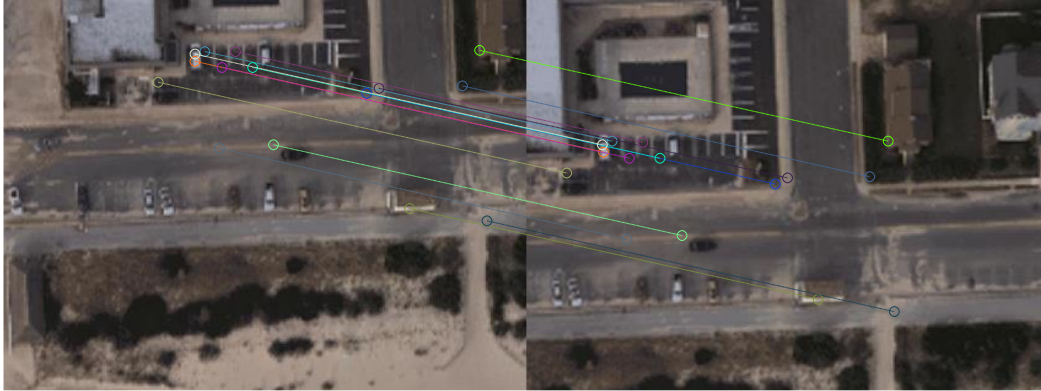
Figure 8: Top SIFT Features identified and correlated between two overlapping images [29] [National Oceanic and Atmospheric Administration, "Hurricane SANDY Response Imagery," National Geodetic Survey, 2012]. Used under fair use, 2014.
