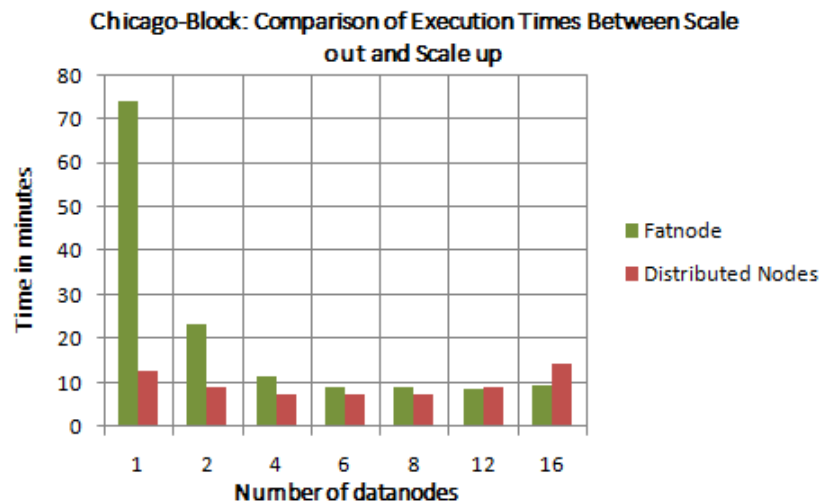
Figure 8.15: Performance comparison of PostgresXC - on a Single Fatnode and Distributed cluster nodes. The plot gives the total running time of Indemics with PostgresXC as the RDBMS. The results are for Block intervention scenario over Chicago region. The number of datanodes are varied from 1 through 16.
