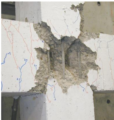
Figure 2.4 Crushing within joint core. Pagni, C., and Lowes, L. (2004), "Predicting Earthquake Damage in Older Reinforced Concrete Beam-Column Joints." Report No. PEER-2003/17 , Berkeley, CA. Photo used under fair use, 2014.
