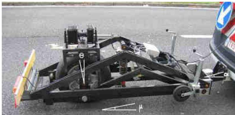
Figure 1 – BRRC trailer with indication of  $\alpha$ ,  $\mu$  and  $\theta$
