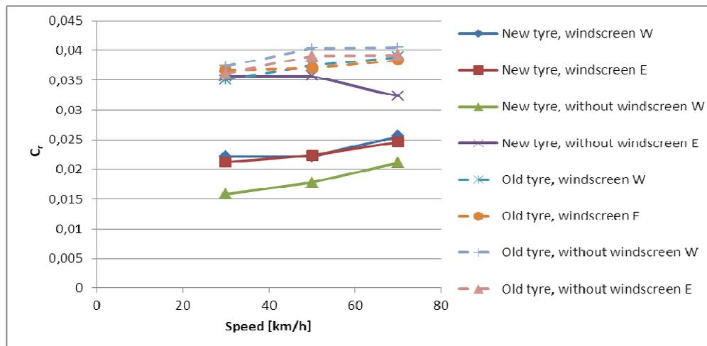
Figure 10 –  $C_r$  as a function of speed
