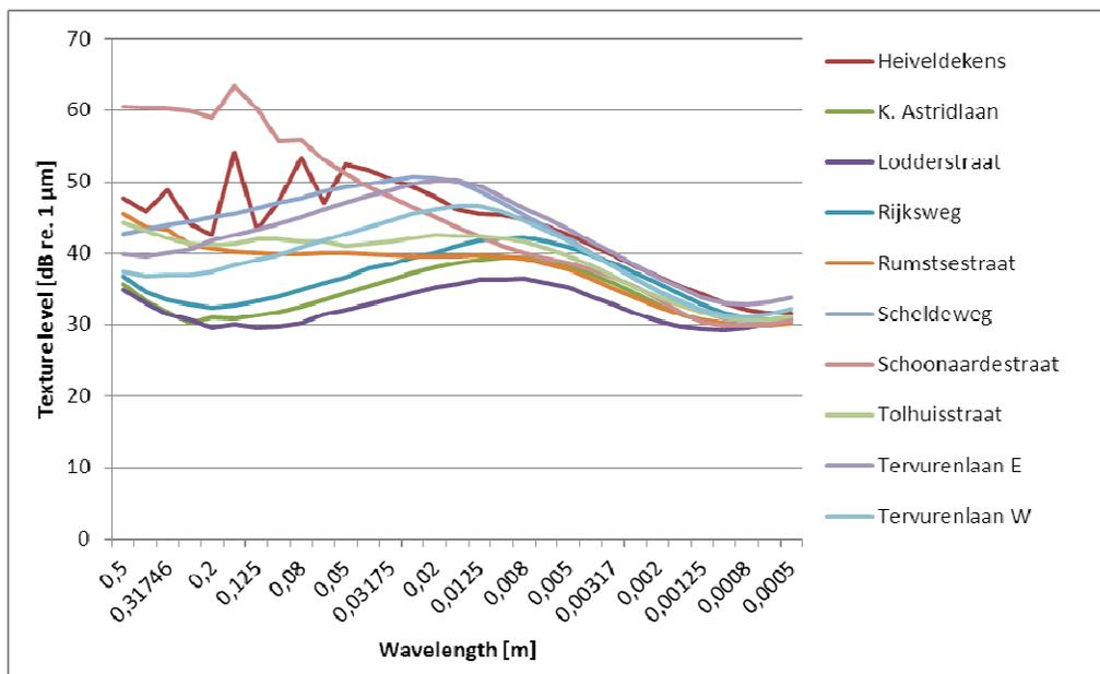
Figure 12 – Overview texture spectra test sections De Bie-Hofmans
