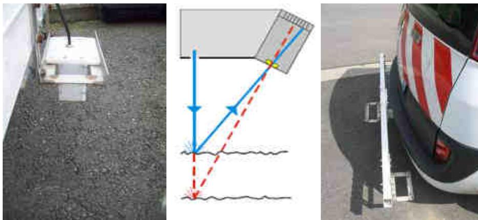
Figure 3 – Dynamic laser profilometer BRRC
