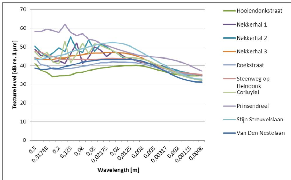
**Figure 13 – Overview texture spectra test sections Aerts-Cools**
