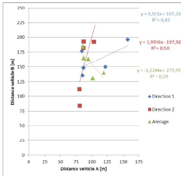
Figure 16 – Correlation between coast down measurements both vehicles – only test sections with similar texture spectra in both directions
