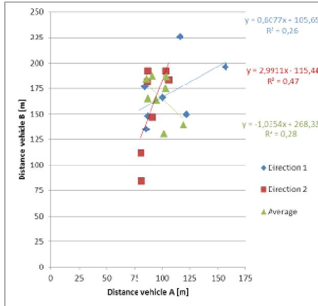
Figure 15 – Correlation between coast down measurements both vehicles – all test sections
