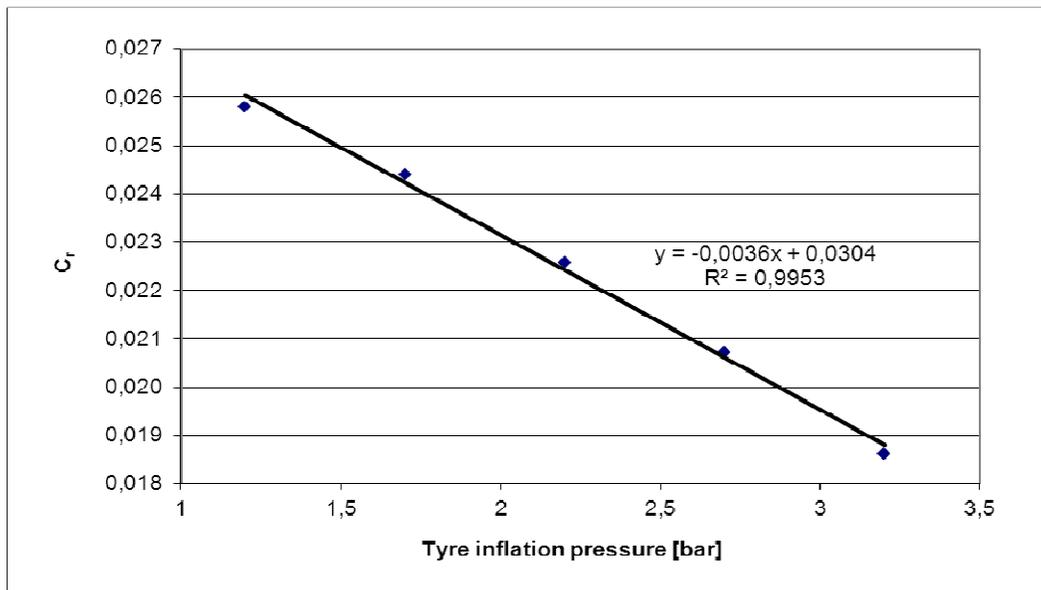
Figure 8 – Correlation between average  $C_r$  and tyre inflation pressure
