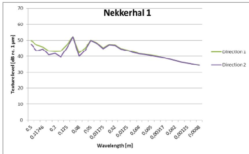
Figure 14 – Texture spectra both measurement directions test section “Nekkerhal 1”
