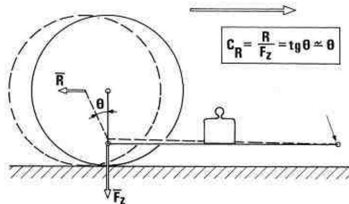
Figure 2 – Measurement principle BIRC trailer
