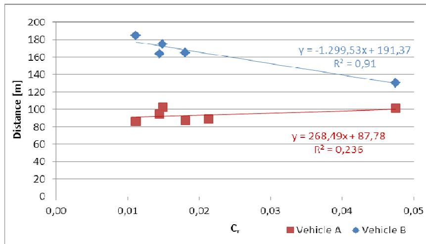
Figure 17 – Correlation between  $C_r$  measured by Dotsenko-Helsen and coast down distance measured by Aerts-Cools
