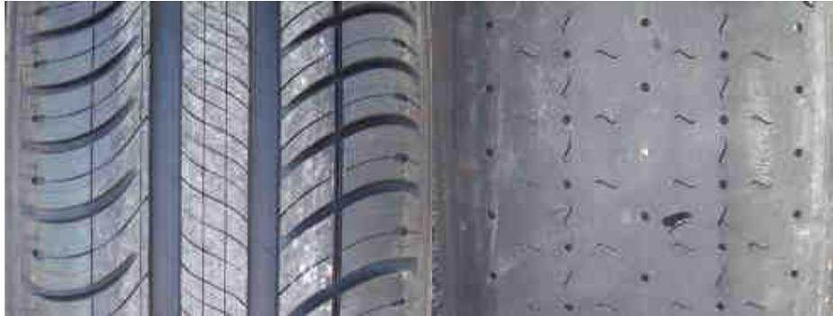
Figure 11 – New Michelin Energy Saver tyre (left) and old Michelin slick tyre (right)
