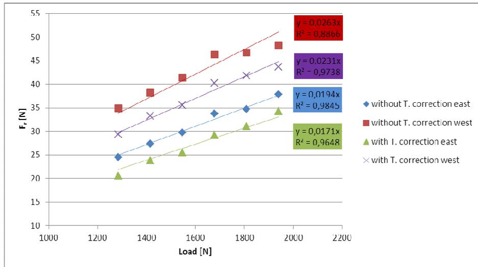
Figure 7 – Influence of vertical load on rolling resistance force
