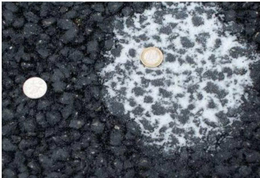
Figure 1 – A Typical Surface Texture of Ungrooved AC-14 BBA D
