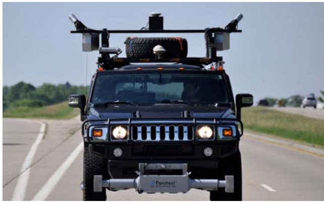
Figure 2 – Multi-function pavement data collection vehicle.
