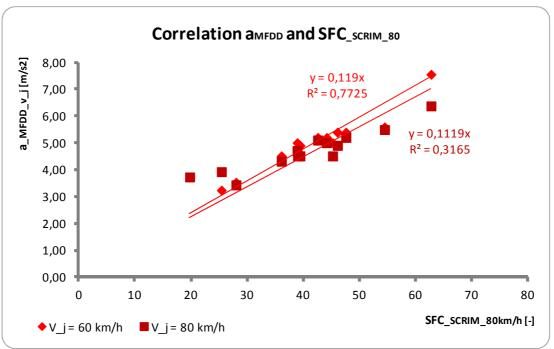
Figure 7 – Correlation for skid resistance at a measuring speed of 80 km/h
