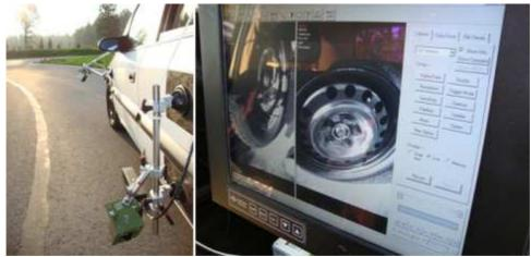
Figure 2 – High speed cameras on a minivan
