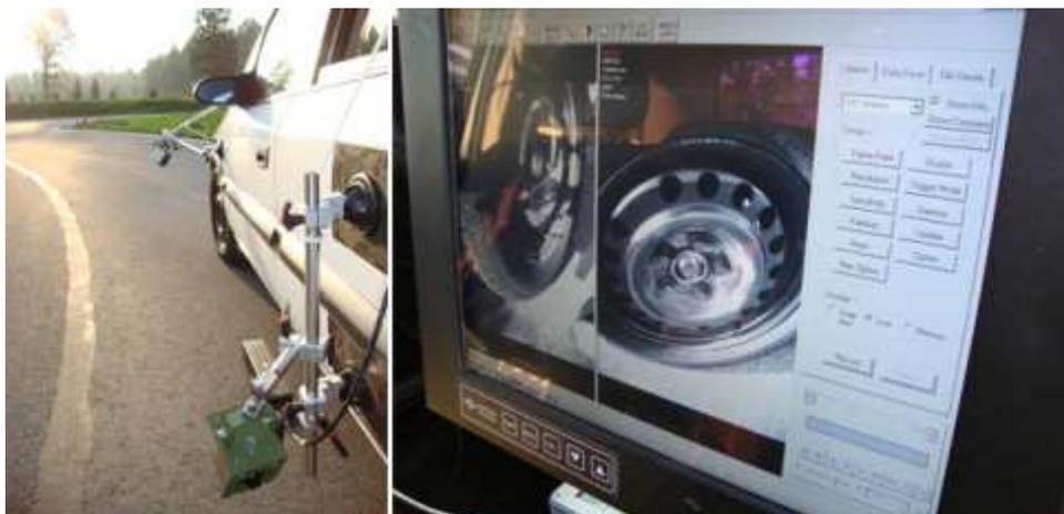
Figure 2 – High speed cameras on a minivan
