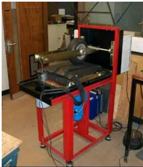
Figure 8 – Test equipment to measure tyre / asphalt contact area / stress
