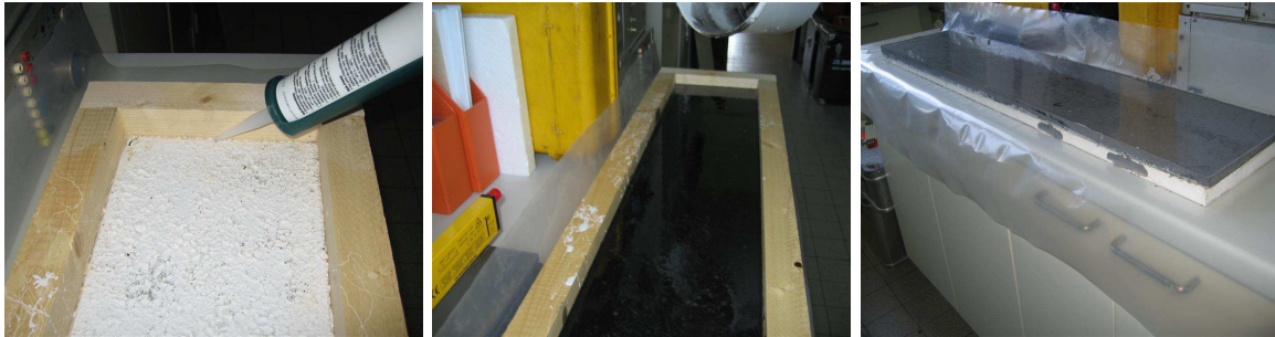
Figure 2 – Making of a positive print in epoxy using the same wooden frame
