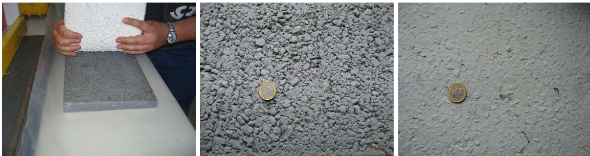
Figure 3 – Removing the mould (left) and the results: a sample with a coarse texture (sample 1, middle) and a sample with a smoother texture (sample 2, right)
