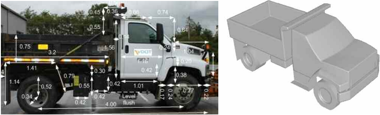
Figure 4 – Digitised photograph (left) and solid model (right) of the dump truck
