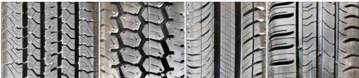
Figure 8 – Tread patterns of the test tyres; from left to right: SRTT, AAV4, ES14 and ES16.
