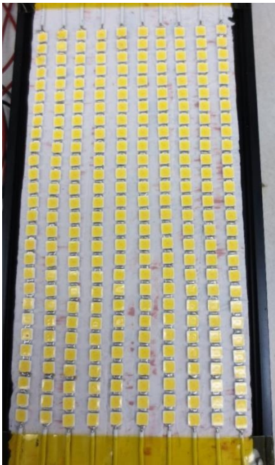
Fig. 5.3. Balanced Load of 2-stage LED driver: 10 LED strings with Cree XLamp MX-3 LEDs
