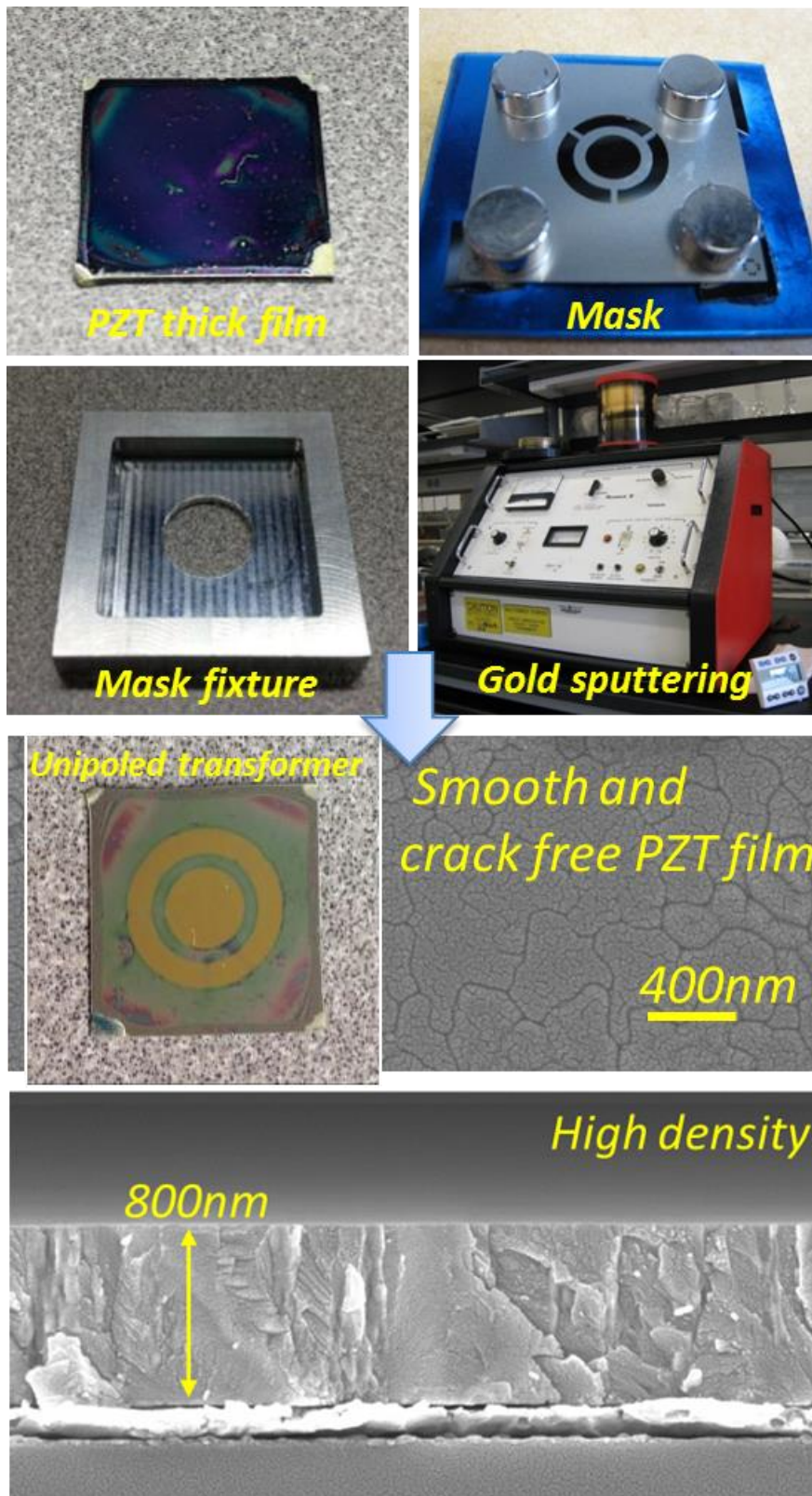
Figure 5.18 Unipoled thin film PZT transformer synthesized by Au sputtering.
