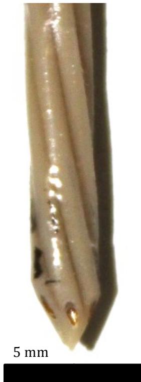
Figure 3-2: Finished distal end of arborizer.
