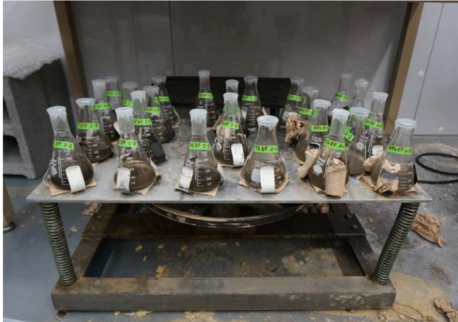
Figure 3.1: Erlenmeyer flasks with 5 g samples and 100 ml extraction fluids placed on a shaker table
