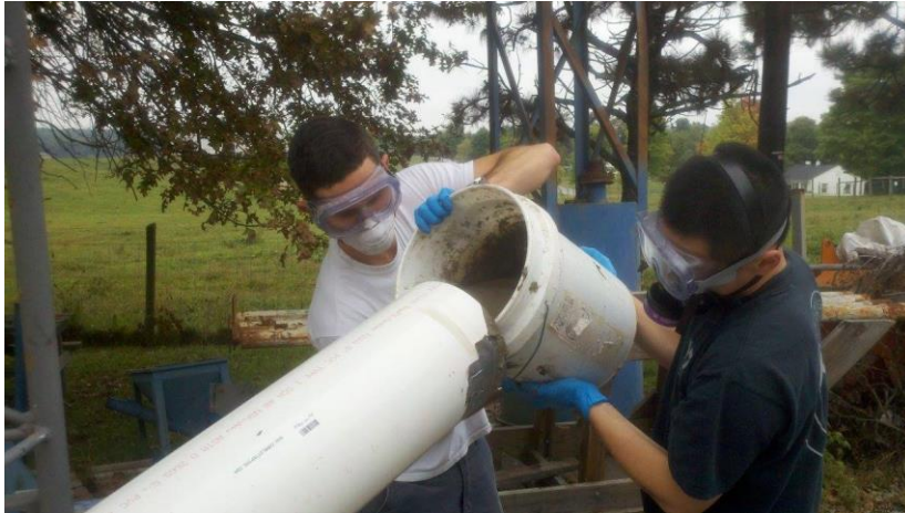
Figure 4-1. Filling of one of the pipes used in the large-scale experiment in Virginia. Photo by author, 2013
