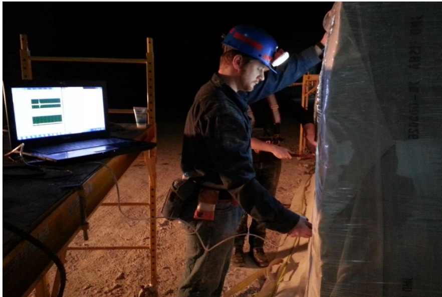
Figure 5-3. Researchers from VT and UK holding the geophone in place and applying the energy source on the full scale seal. Photo by author, 2014
