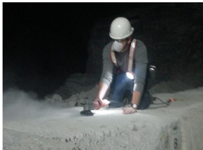
Figure 5-2. Grinding smooth surface for geophone placement on top of the large scale samples. Photo by author, 2014
