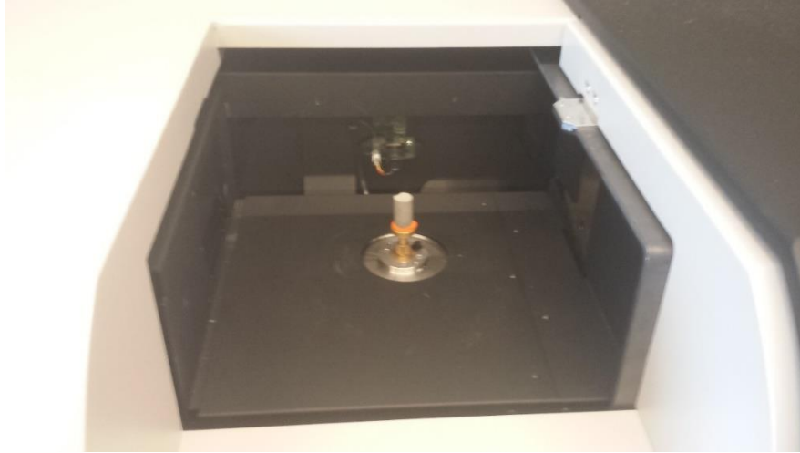
Figure 6-7. Seal sample in the SkyScan 1172. Photo by author, 2014
