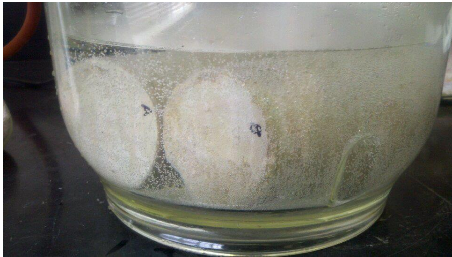
Figure 6-2. Seal material samples during effective porosity test. Photo by author, 2013
