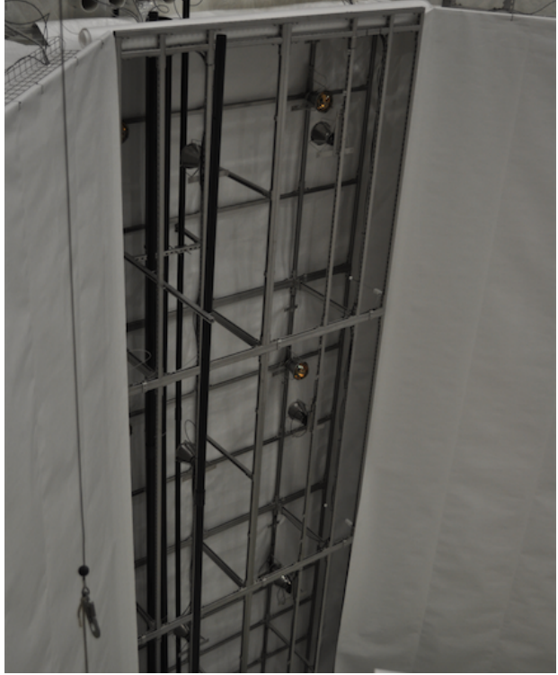
(b) Partitioning with Tyvek. PMT shown in OWS.
