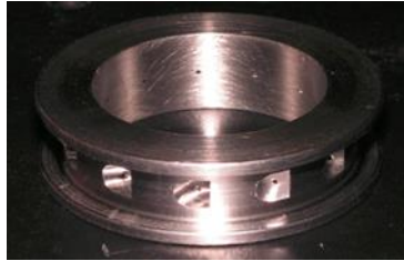
Figure 2.14. Machined fuel block (12-18T). Photo by author, 2012.
