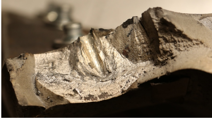
Figure 3.51 – Close-Up of Fracture Initiation Location at Outer PAF
