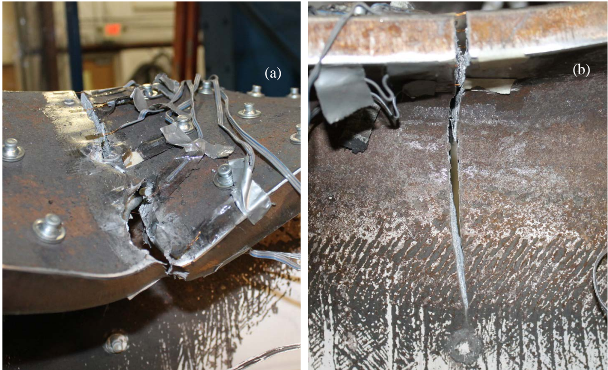
Figure 3.49 – Pictures of Final Top Flange Fracture for Specimen 9 (W36x150 with RBS and Grid of PAF)
