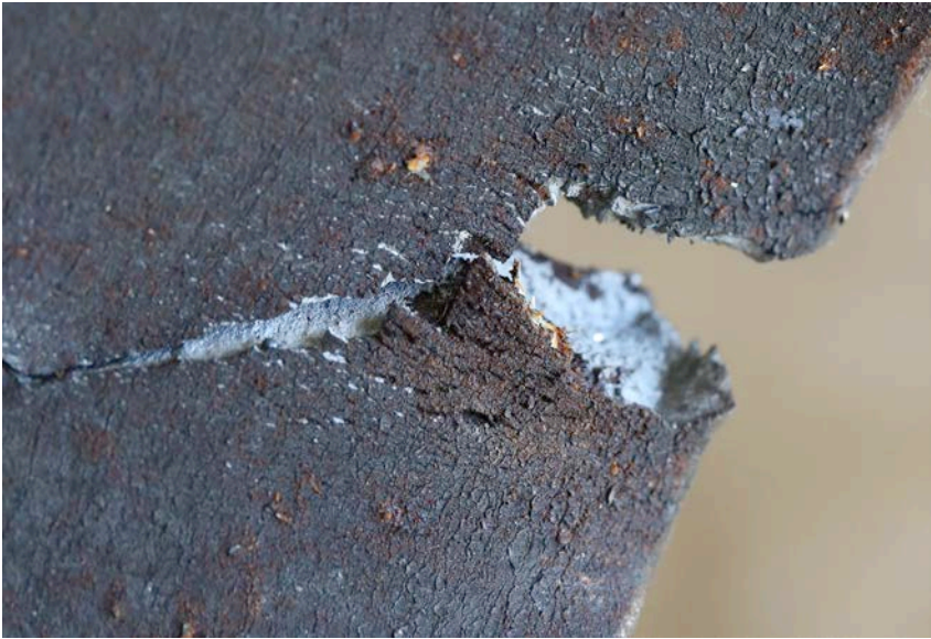
Figure 3.6 – Flange Surface of Fracture Propagation
