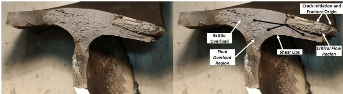
Figure 3.38 – Fatigue Crack Propagation Starting with Crack Initiation Followed by the Critical Flow and Final Overload Regions
