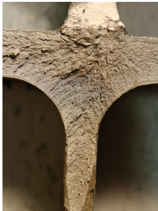
Figure 3.44 – Close-Up of Chevron Markings at the Web and Flange Pointing Back to the Fracture Origin at the Weld Metal of the Stiffener Due to the Brittle Overload Fracture Mode
