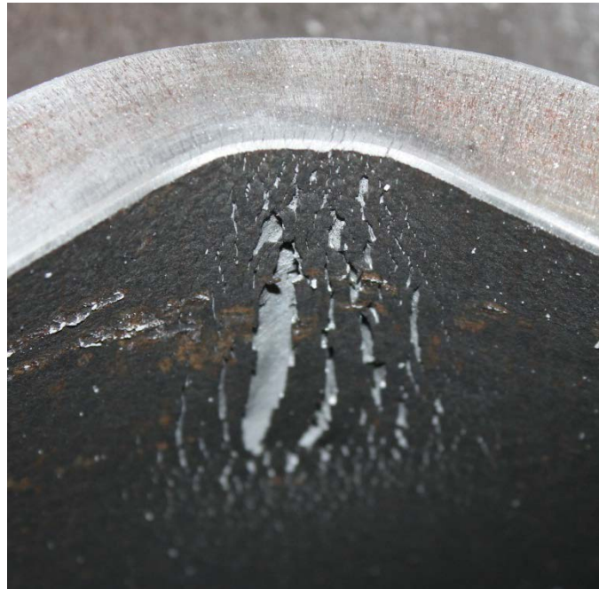
Figure 3.35 – Crack Initiation on Surface of Bottom Flange for Specimen 7 (W36x150 with RBS and No Fasteners)
