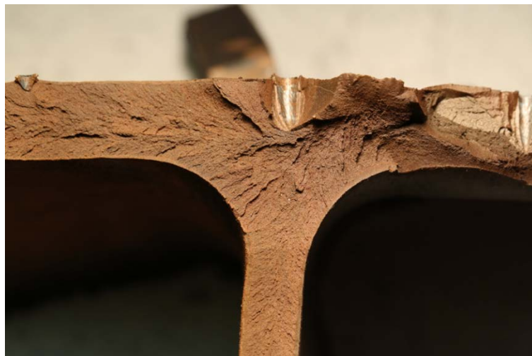
Figure 3.66 – Close-Up of Chevron Markings at the Web and Flange Pointing Back to the Fracture Origin at the PAF Due to the Brittle Overload Fracture Mode
