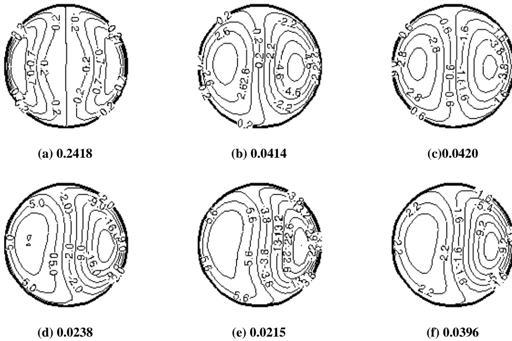
Figure 5.5 Secondary flow patterns at 44a from inlet of helical tube at six time values (a) T = 0.0 (b) T = 1.05 (c) T = 2.1 (d) T = 3.15 (e) T = 4.2 (f) T = 5.25 . The values below the figures are the non-dimensional parameter \gamma as defined in Eq. (13). The helical tube is stationary.
