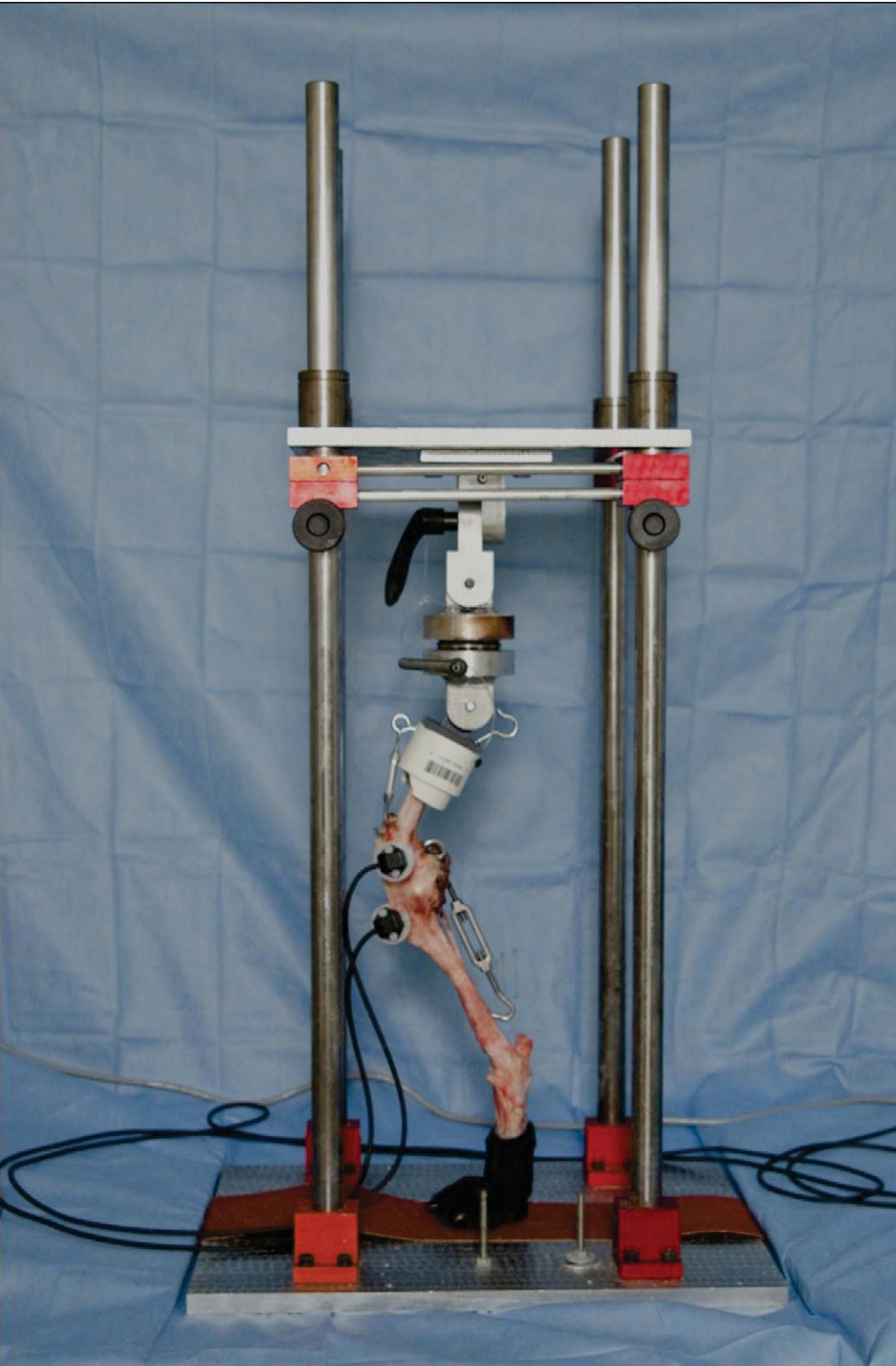
Figure 12: Loading frame. Biomechanical testing setup with the limb secured into the loading frame and femoral and tibial sensors in place.
