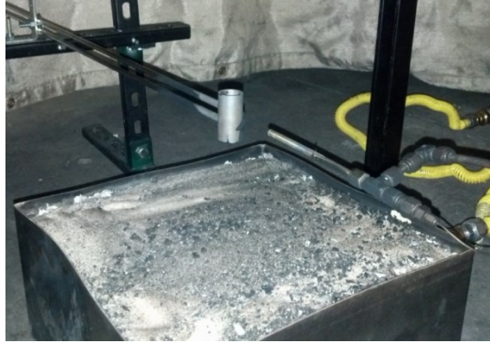
Figure E.5: Bi-directional and Aspirated Thermocouple Probe Placement
