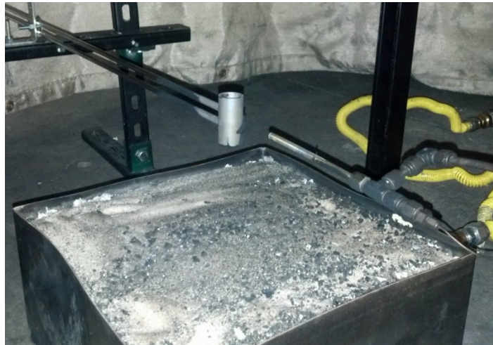
Figure D.4: Bi-directional and Aspirated Thermocouple Probe Placement
