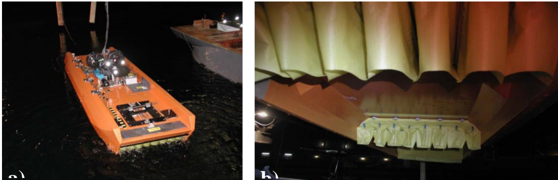
Figure 8 - NSWCCD Model Number 5887, generic T-Craft SES model with finger type bowl seal (left). A view of the underside of the craft showing the bow seal, transverse mid-cushion seal, and stern seal (right) (12).
