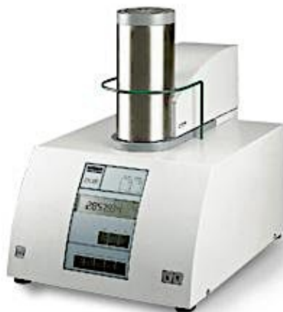
Fig. 4-2. Simultaneous thermal analyzer NETZSCH STA 449 Jupiter.
